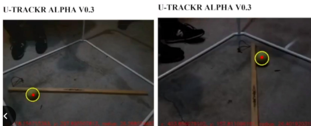
Figure 6. Object Recognition: The tested tennis ball has a defined XY coordinate system with respect to the image frame. The set radius of the ball is defined.
