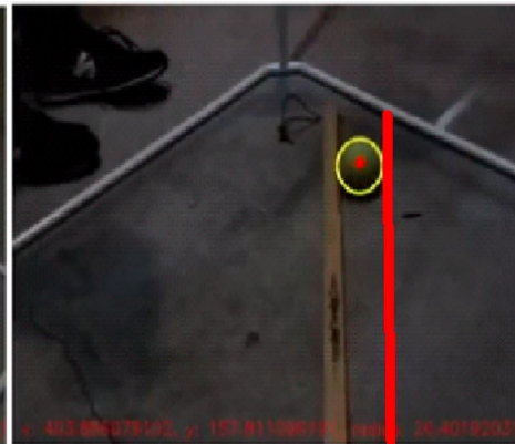
Figure 11. Epipolar Geometry of Tennis Ball Feature: Red line indicating the epipolar line.
